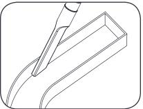
Before you begin, clean surfaces and remove all debris from the inside of the channel letter. Clean the surfaces with a 50:50 mixture of isopropyl alcohol (IPA) and water and let dry.
