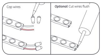
Must cap all exposed wires with appropriate wire connectors and seal with electrical grade RTV silicone.
