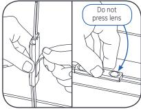
3 Remove tape backing and stick LED modules into place. When using tape apply approximately 15 psi pressure on the module (avoid the lens dome surface) for 5 seconds, full bonding strength after 24 hours. Continue until you have reached the end of the strip.
