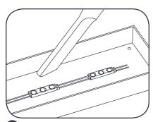
6 Remove all debris from the inside of the channel letter and replace the sign face.
