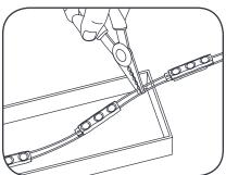
Measure and cut Select LED strip to the appropriate length for each letter. Cuts can be made between any of the modules.
