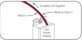
3 Run a wire from the LED Power Supply to each channel letter and connect to the first LED module on the strip.
