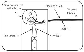
4 Connect the red stripe wire (+) of the LED strip to the red wire (+) of the power supply. Connect the white wire (-) of the LED strip to the black or blue wire (-) of the power supply.
