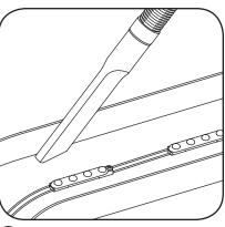
6 Clean and remove all debris from the inside of the channel letter. Replace sign face.
