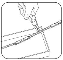
2 Measure and cut Tetra LED strip to the appropriate length for each letter. Cuts can be made between any of the modules.
