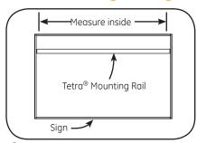
Measure and cut Tetra® Mounting Rail or other suitable mounting means to appropriate length to fit into sign.
