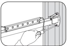
Secure the Mounting Rail to the inside of the box sign using a Tetra® Mounting Rail Clip or other suitable mounting means. Ensure the #6 (M3) screw does not exceed 3/4 inches (19 mm) in length.
