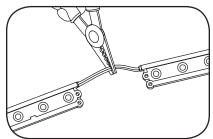
2 Determine how many modules are required for one row and cut wire.
