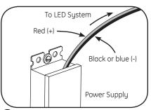
Run a wire from the power supply to inside the sign and connect to the first module on the strip.
