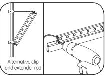
Arrange modules evenly spaced apart. Place the Tetra® modules on the Mounting Rail and secure into lip with a self-tapping #6 (M3) screw or 1/8-inch (3.175 mm) rivet. Or mount using the alternative clip and extender rod configuration.
