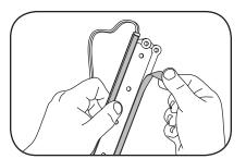
Peel off backing to expose adhesive tape.
