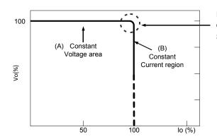
Typical LED power supply I-V curve
