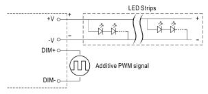
"DO NOT connect "DIM- to -V"
