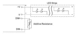
"DO NOT connect "DIM- to -V"
