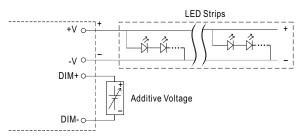
"DO NOT connect "DIM- to -V"
